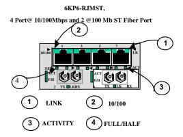
port supports fiber optic cable distances up the IEEE-standard 100Mbps distance limits, i.e., typically 2km at full-duplex and 412m at half-duplex.
